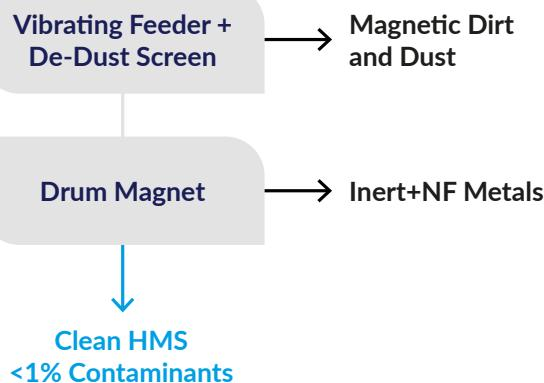
Part of the contamination in scrap is made of non-ferrous magnetic dirt and dust.
